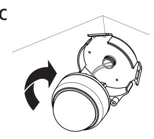
Fit and tighten the dome camera on the coner mount by rotating clockwise.
